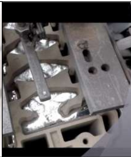
Gas formation during casting
