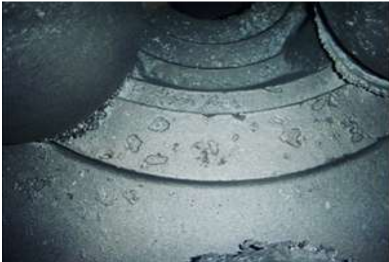
Casting defects caused by fiber sleeves
