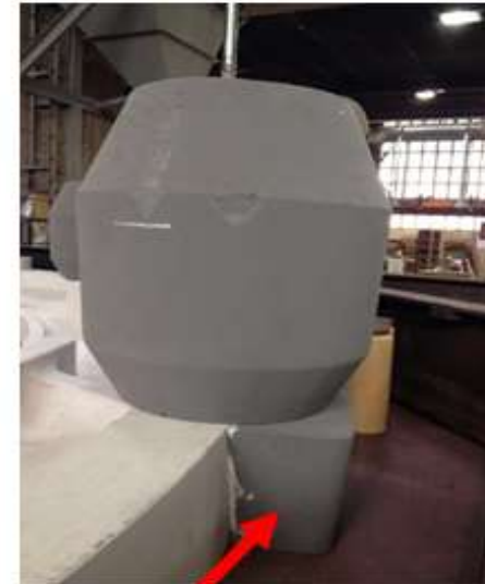
EXOTHERMIC PADDING Applied as a separate core
