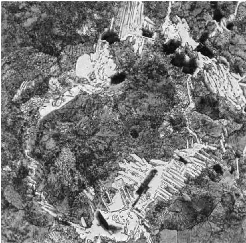
Intercellular Carbides in a 7,62 cm diameter Ductile Iron bar containing 0,4%Mn and 0,2% Cr; it is worth noting that the effects of Cr and Mn on carbide formation are synergetic, not simply additive!
