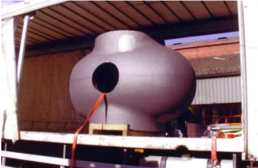
Hub for wave energy generator (9 tons)
