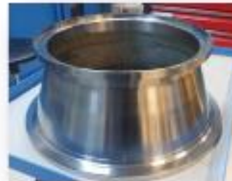
Near Finished Component with 1.5:1 Buy to Fly vs. Up to 10:1
