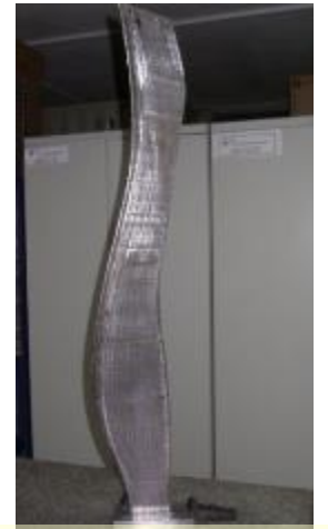
42" Ti64 MLE built at TTC under IMPALA program
