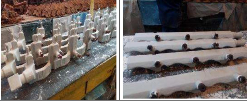
Cores dipped in Solitec IM 801 followed by Miratec TS 405
