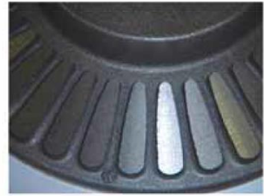
RP 65 AFS GFN + 5 % ESA 2011, 1.7 % cold box binder, without coating
