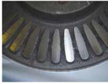
RP 55 AFS GFN + 5 % ESA 2011, 1.5 % cold box binder, without coating
