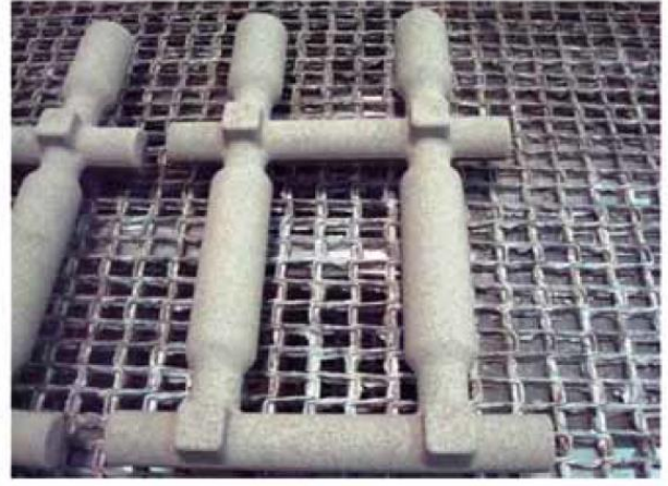
Cardian Joint with 70 AFS GFN sand + 5 % ESA 2011 - cold box core weight of the piece: 2.8 kg., thickness: 35 mm., vertical molding line 450 mm ferrostatic pressure
