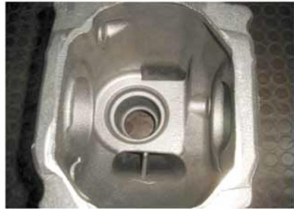
55 AFS GFN sand + 5 % ESA 2011, without coating - 1.5 % cold box 419/619
