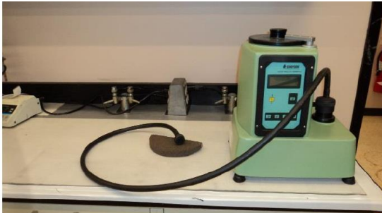
Fig. 5. Core permeability was measured with the unit shown above.
