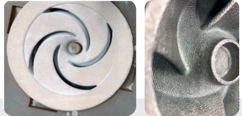
Printed Impeller on S-Max Printer
