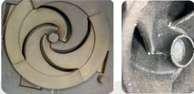
Impeller Core via Core shooting machine
