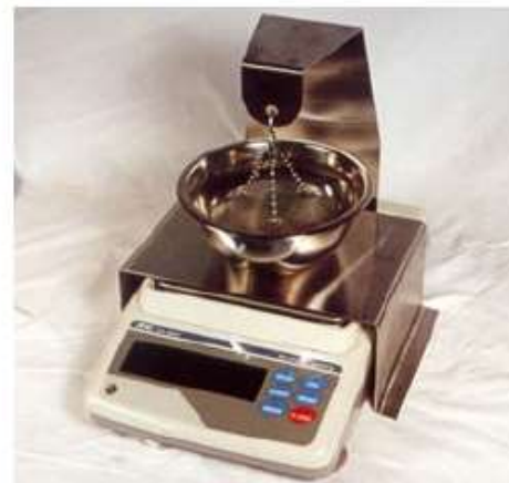
simple system for specific gravity measurement
