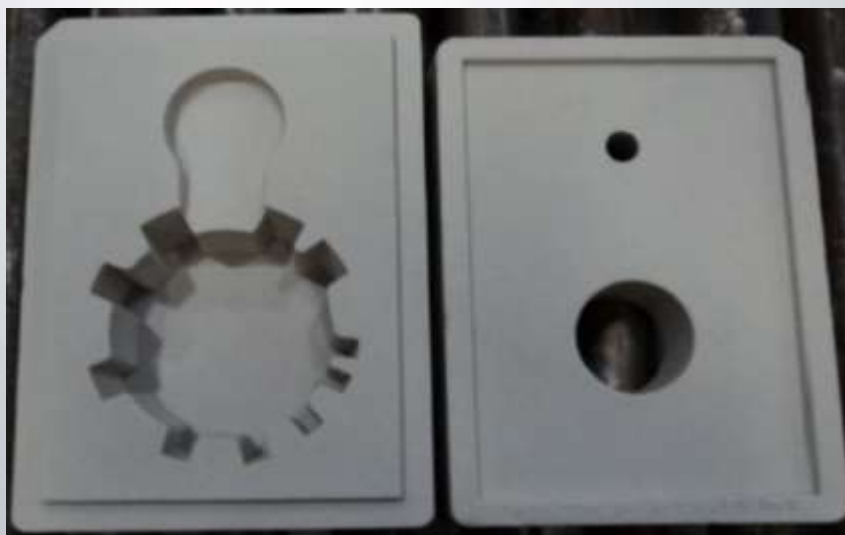
Fig. 1: Using the Hoodstack method with small irregular gear tooth mold
