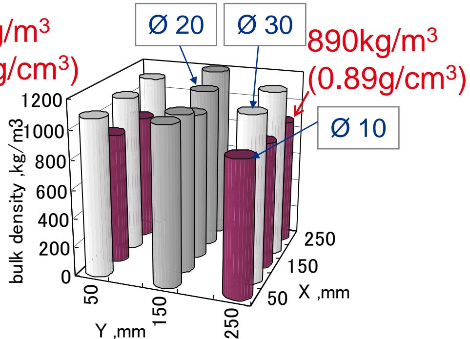
High pressure filling of green sand has an energy loss and an opposite effect for filling into the small pocket.
