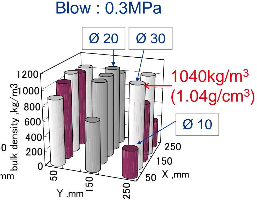
Bulk density : 1,000 kg/m<sup>3</sup> before molding at CB40%
