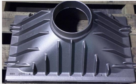
Fireplace roof casting
