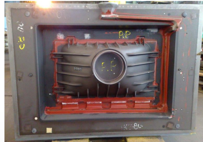
Fireplace roof placed into DISA bolster
