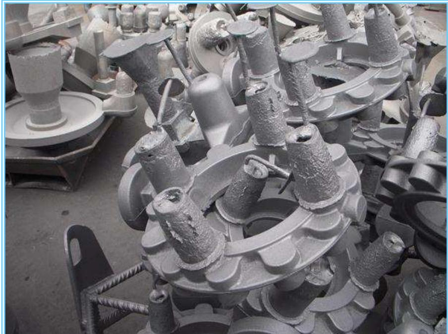
**SS VALVE CASTING WITH FIBRE SLEEVES
