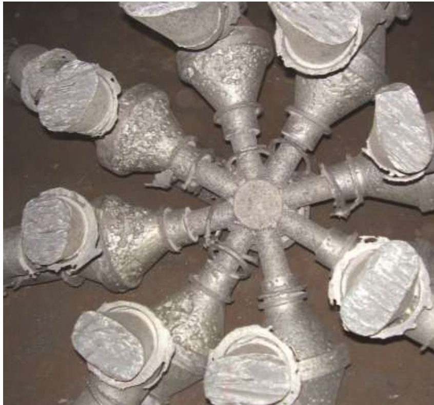
Effective slag retention by filters
