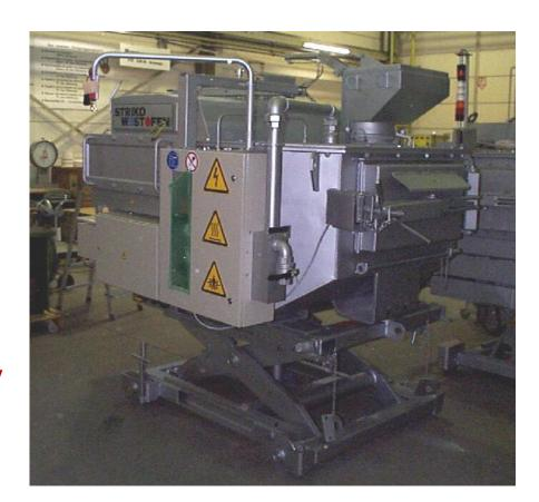
**Porous plug technology** for molten metal processing in the dosing furnace.
