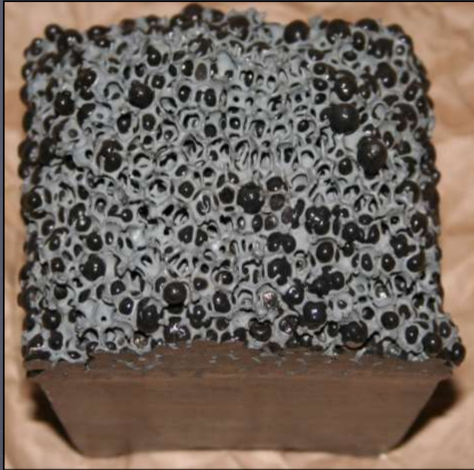
Fig. 3a : "Blocked Filter". View from below.
