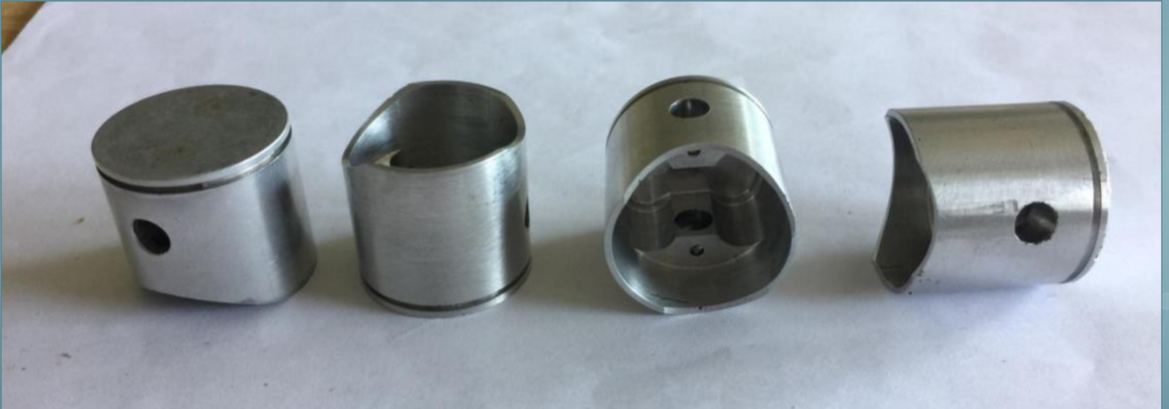
Figure 12. Pistons after squeeze casting and machining.
