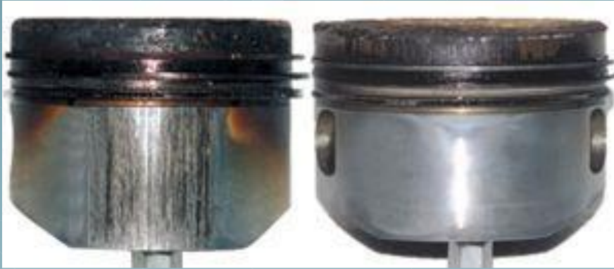
Figure 8. The example of damaged pistons[10]. Comparison of Wear and New Pistons, Retrieved April 2018 from http://www.protectivecoatingsystems.com/zmax
