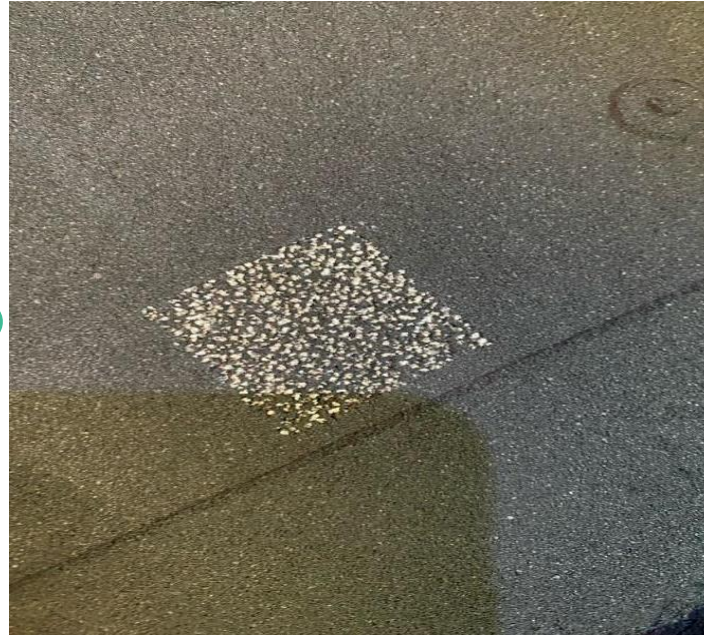
CDOT code first trial with 50 Watt laser with 300mm lens
