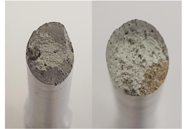
Fracture Surfaces of Specimen 3 and Specimen 6
